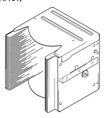
Fitted with a knob which is used to release the locking mechanism, these magazines are convenient for importing or exporting large volumes of discs into or from the changer.
